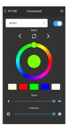
3. If necessary, you can adjust the LED settings to adjust for different types of strips/halos. By default the app & controller should be set to GRB & SK6812-RGBW.
